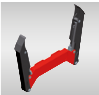
SFD38 flap down stabilizer loose M24, property class 12.9, 42 Cr Mo 4v, locking torque 450 Nm
